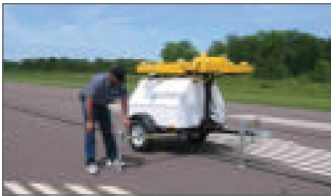
1. Level as necessary using 4 leveling jacks
